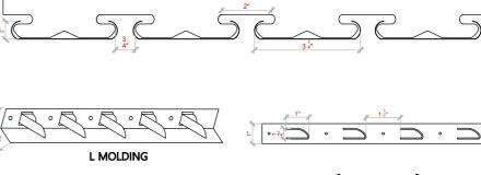
**Physical Data** Galvanized steel - thickness 0.019"
