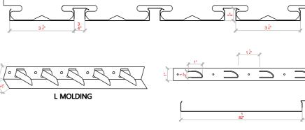
**Physical Data** Galvanized steel - thickness 0.019"
